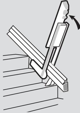
When you are at the bottom of the stairs, you will need to move the stairlift back up the stairs so that the hinged rail does not obstruct any doorway or passageways. This will also make sure that the stairlift is on charge.
